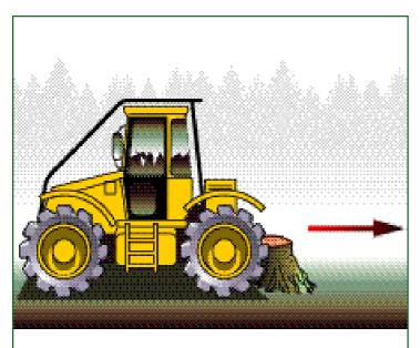
Figure 1 Stump used as anchor
