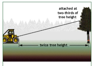
Figure 3 Attachment point for directional felling
